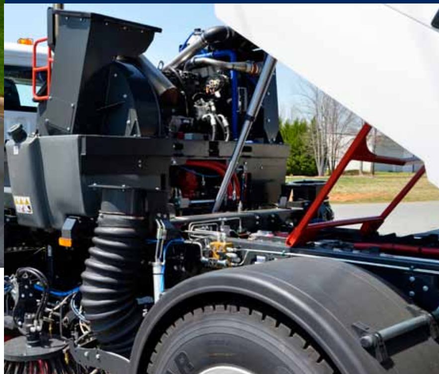
ABOVE Stainless steel hydraulic lines, wider blower intakes, and new improved body safety prop automatically deploys.
