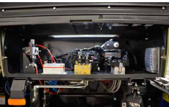
Accessible systems locker with LED service light.
