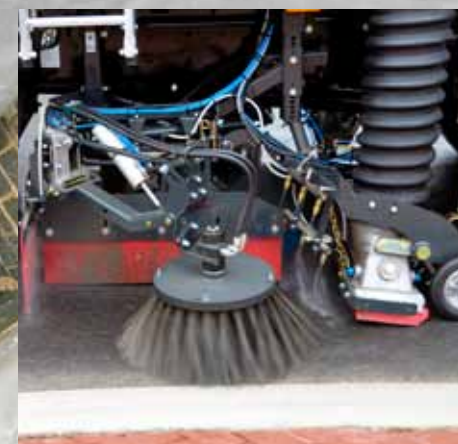
Variable lateral control Varibrush option.
